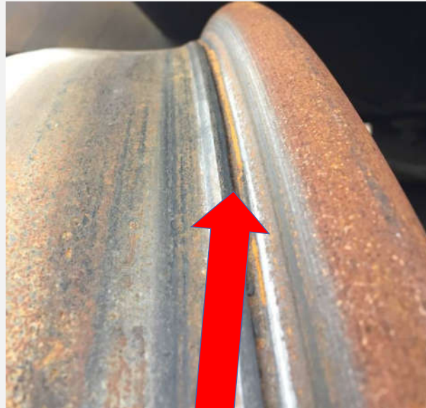
Extraordinary wheel tread deformation near the flange
