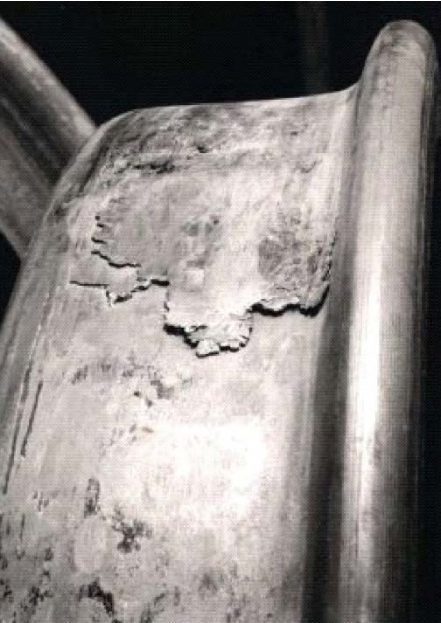
Metal build up on the tread
