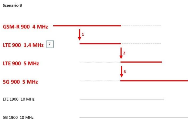
Figure 25. Migration scenario B: keeping GSM-R while introducing 1.4 MHz LTE in 900 band
