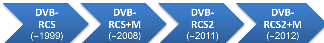
Figure 40: Evolution of the Return Channel via Satellite
